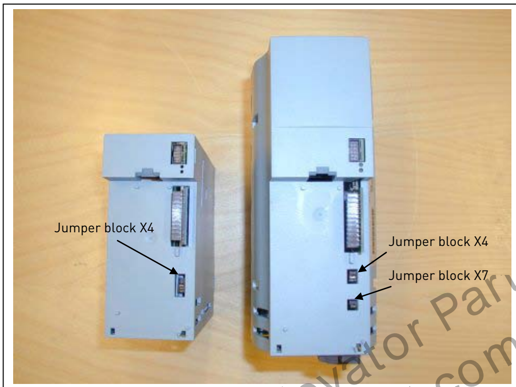
Figure 6-25. The location of jumper blocks in MF2 (left) and MF3 (right)
